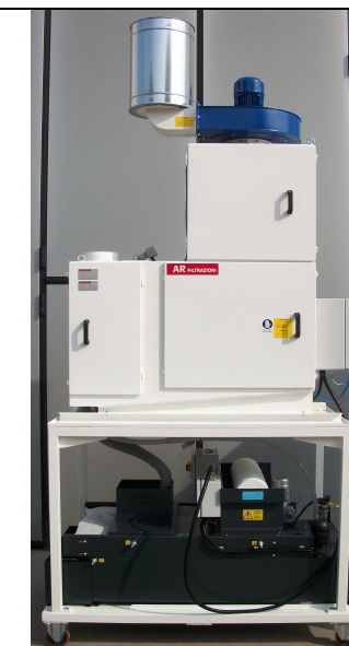
SERIE HYDROFILTER CON SILENZIATORE E VASCA HYDROFILTER SERIES WITH NOISE ATTENUATOR AND TANK
