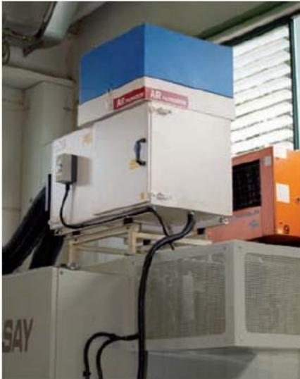
**An AR air cleaner of the ARNO series installed on an automatic lathe**
