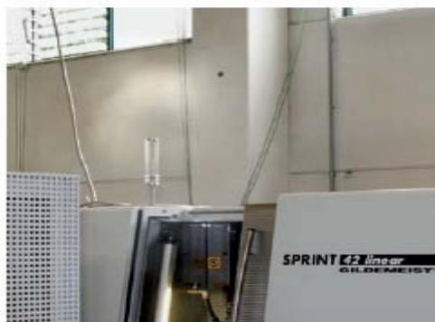
**A machine tool working with the air cleaner deliberately turned off: you can see clearly the emission of whitish oil mist. In these conditions, with tens of machines tools up and running in the workshop, the working environment would quickly become unhealthy.**
