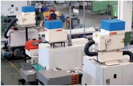
**Another image of the workshop of OMZ. The air cleaners of AR Filtrazioni can be seen. Oil mist and smoke have completely disappeared.**
